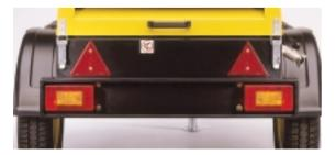
Recessed into the rear chassis rail for protection, the road lighting system comes as standard.
