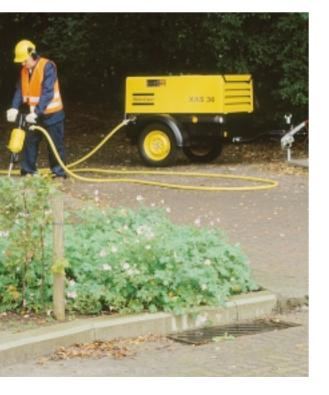
Both compact and light, the XAS36 does not need have brakes and can be towed by a car. Designed to be stable at high transport speeds, the compressor is also offered with a choice of towbar.
