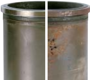
The engine liner on the right, using a conventional coolant, reveals severe cavitations pitting and corrosion. The one on the left shows no defects after the same number of operating hours with PARCOOL EG .
